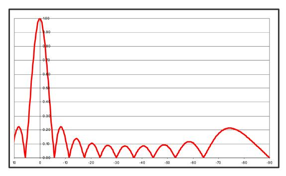
The plot below is the same 10 bay antenna, operating at channel 11. The spacing at channel 11 (198 – 204 MHz) is more than the  $1\lambda$  spacing used at channel 7
