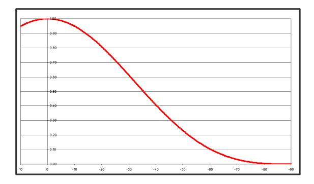
The suppression of this pattern is so good at high depression angles that the radiated power is only 45 mW at those angles. That is almost 40 dB of suppression! Between good bonding of the antenna and using an all stainless steel antenna welded design, PIM generation is not likely to happen. If questions come up about mounting your new Micronetixx LPFM antenna, please let us know. We are happy to help out.
