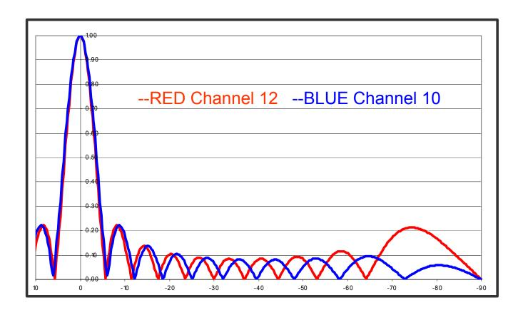
Now let's shorten up the antenna even more. We will space the antenna at  $7/8\lambda$  (or 315 degrees) on channel 12. The spacing will reduce to  $0.82\lambda$  (296 degrees) on channel 10. This antenna will be 13-7/8 feet (4.22 meters) shorter than the stock channel 7 to 13 design. The elevation gain has dropped slightly to about10 (10.00 dB) on channel 12 and 9.6 (9.82 dB) on channel 10. The off the shelf 10 bay bat wing had a gain of about 9.7 (9.86 dB) on channel 10.
