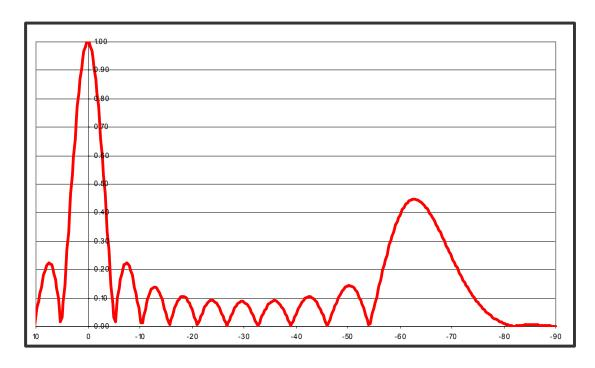
The gain of the batwing at channel 7 is about 10.5 (10.21 dB, while the gain at channel 11 is about 9.5 (9.77 dB). The increased spacing between bays and the formation of the large grazing lobes decreases the array gain.
